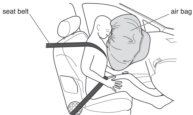
The airbag and seatbelt change shape and absorb energy in the crash.
